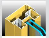
All 424 framing is designed to accept IGUs up to 28mm.
